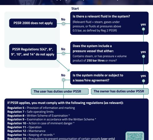
This decision tree only applies to type (a) pressure systems as defined in Regulation 2(1) PSSR: one or more pressure vessels of rigid construction, any associated pipework and protective devices.
